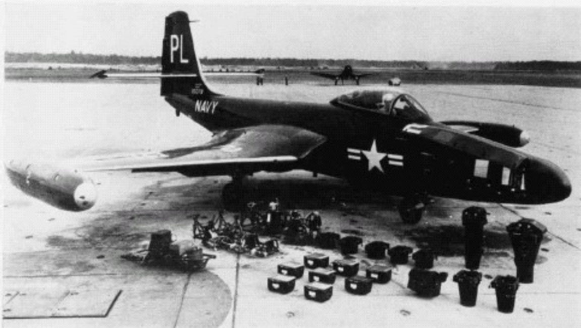
INSTALLED IN THE PHOTO-SANSHEE'S NOSE, THESE AERIAL CAMERAS CAN MAKE DAY OR NIGHT, OBLIQUE OR VERTICAL PHOTOS
